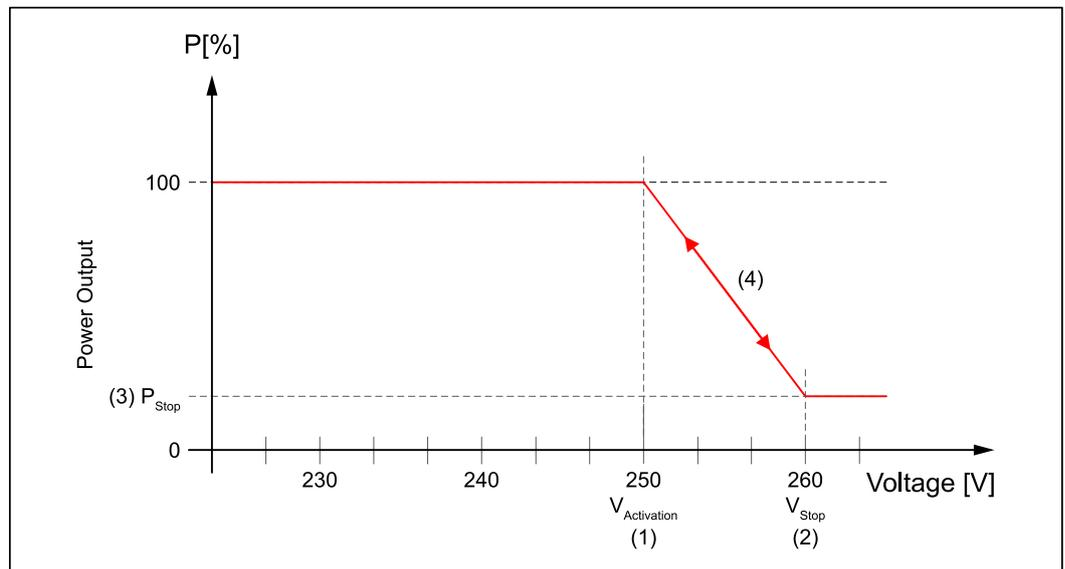
Power curve when "Activation Threshold Overvoltage" is exceeded.
