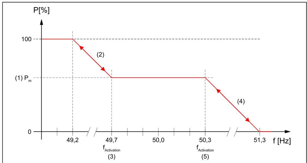
General power curve with overfrequency and underfrequency without hysteresis with gradients.
