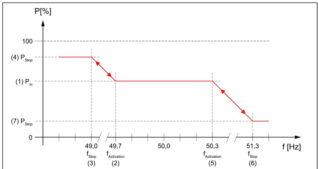
General power curve with overfrequency and underfrequency without hysteresis with stop frequency.
