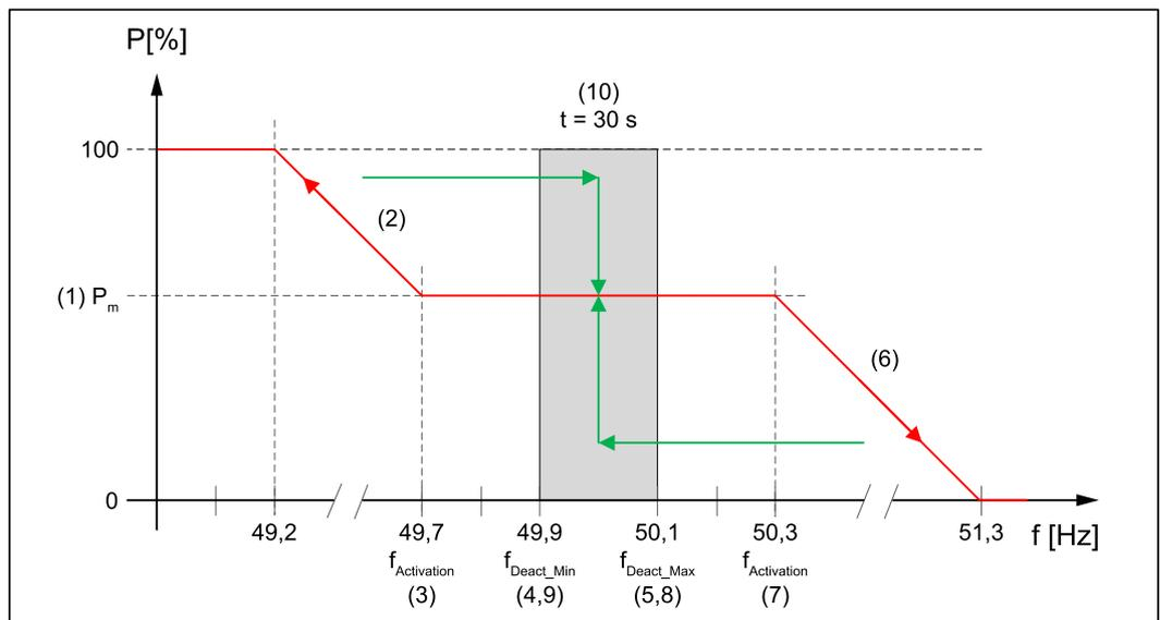
General power curve with overfrequency and underfrequency with hysteresis with gradients.
