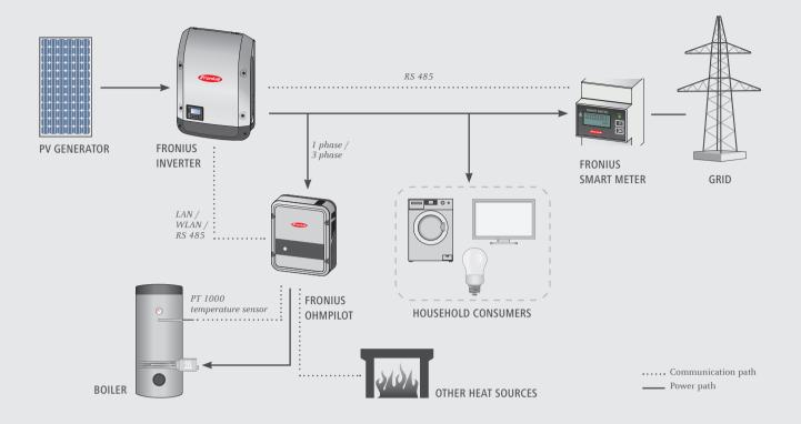
Installing the Fronius Ohmpilot could not be easier thanks to straightforward commissioning via the dedicated website as well as a simple communication connection via WLAN. The Fronius Ohmpilot also protects the grid by cleanly and reliably activating the consumers, leaving you as the installer fully equipped for the demands of today and tomorrow. When using 3-phase heating rods, ensure that the neutral conductor is connected to the input voltage and the heating rod.
