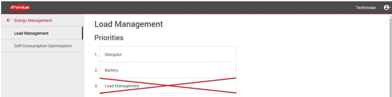
**Fronius does not recommend using the digital I/Os and the Fronius Wattpilot at the same time, as the loads cannot be prioritized.**
